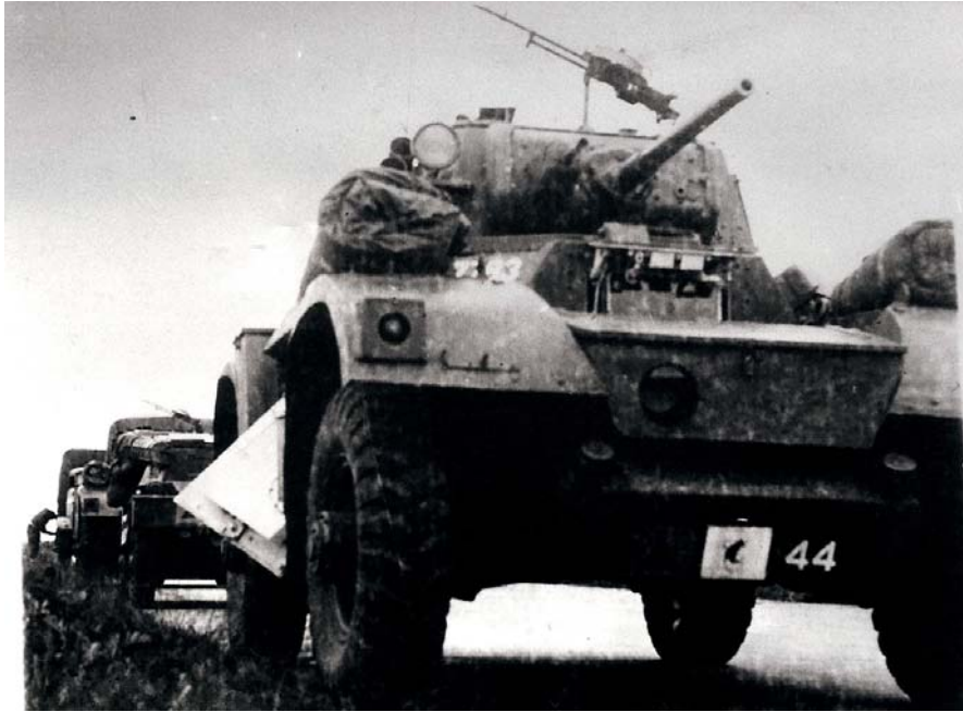
pictures courtesy Martyn Tasker (unknown source) A Daimler Armoured Car of 11Hussars,, again the Vickers K gun is prominent upon its pintle mount on the top of the turret. Circa 1944
